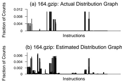
Figure 5: Instruction execution distribution across address range for 164.gzip (a) actual and (b) PMU.
