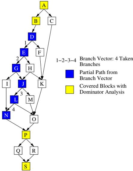
Figure 1: HPM partial path creation and path extension based on dominator analysis.
