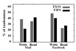
Figure 3: **Percentage random I/O at block level**. This graph shows that the percentage of random writes in F2FS is  $1.5 \times -2 \times$  lesser than ext4, where as F2FS does more random reads compared to ext4.
