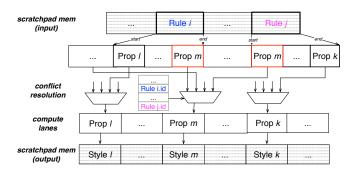
Fig. 10: SRU coupled with scratchpad memories.
